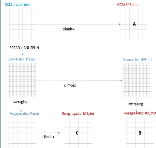
**Figure 2:** Experimental design for downscaling R95ptot index from coarse Global Climate Model (GCM) resolution using the BCCAQ statistical downscaling method and ANUSPLIN target dataset.
